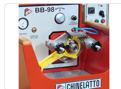
Clamping system with yellow fixture for connecting rods in BB-98 Chinelatto diamond honing machine
