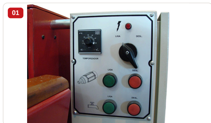
Detail — Control panel of BB-98 honing machine with timer and on/off buttons for operation
