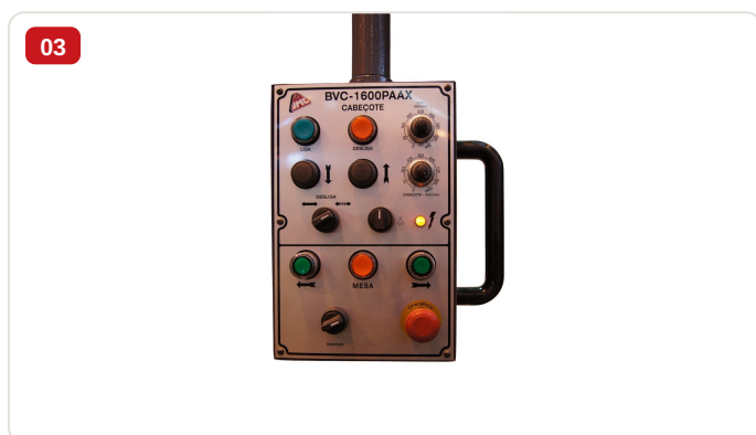
Detail — BVC-1600PAAX control panel with on/off buttons and graduated knobs for boring machine
