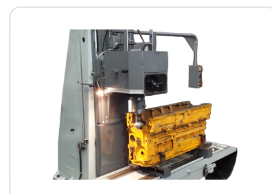
Cast iron engine block being milled on BVC-1600X cylinder boring machine by Chinelatto
