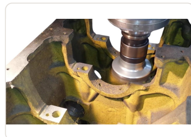
Cast iron engine block being milled on BVC-1600X milling machine with rotating cutting tool
