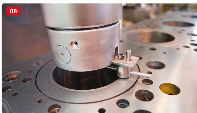
Standard accessory — Centering device with holes for workpiece fixation on BVC-1600X boring machine Chinelatto
