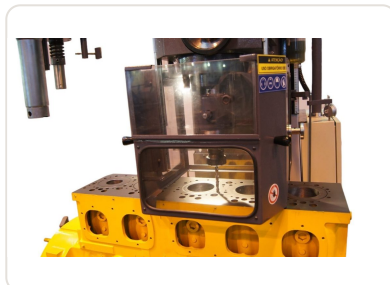
Fixture table with multiple holes for workpiece positioning on BVC-1600X boring machine
