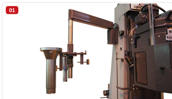
Standard accessory — Boring head of BVC-1600X machine with tool holder spindle and installed boring tool
