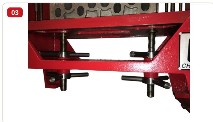
Detail — Height adjustment handles for cylinder head with precision threads on EMC-2 boring machine
