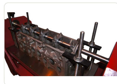
EMC-2 Valve Guide Boring Machine Chinelatto — detailed view of head with tool holder bar
