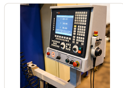
Standard accessory — FAGOR CNC control panel with coordinate display and keypad for FP-3000 portal milling machine
