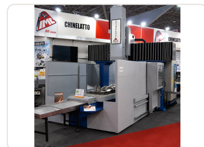
CNC portal milling machine FP-3000 Chinelatto with cast iron structure and 118x39 inch table
