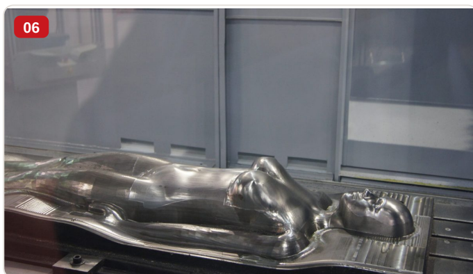
Detail — Cast iron metal part being machined on FP-3000 portal CNC milling machine
