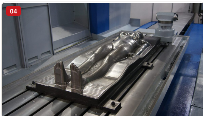
Detail — Machined aluminum mold with human figure cavities on CNC portal milling machine FP-3000 table
