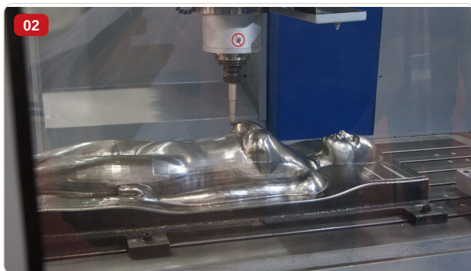
Detail — Metal workpiece being machined on FP-3000 portal CNC milling machine with active coolant
