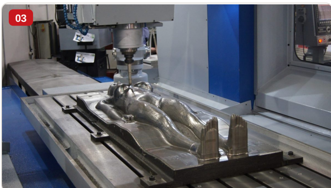
Detail — CNC portal milling machine FP-3000 machining cast iron mold with human figure in relief on table
