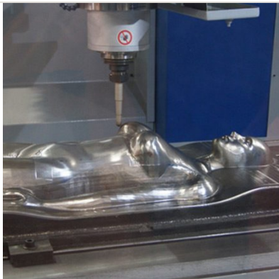
Detail — CNC portal milling machine FP-4000 machining complex metal part with 157x87x35 inch travel
