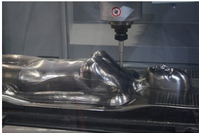
Detail — Complex metal part being milled on CNC portal milling machine FP-4000 CM during industrial operation
