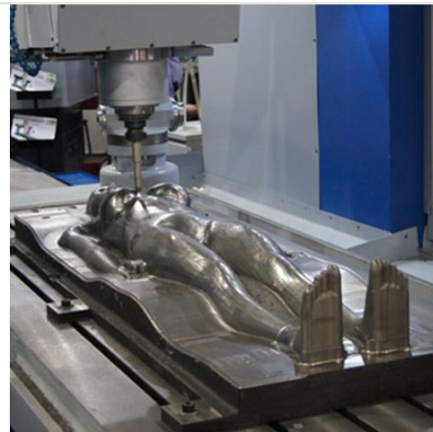
Detail — Sculptural mold machining on CNC portal milling machine FP-4000 with 157x47 inch table
