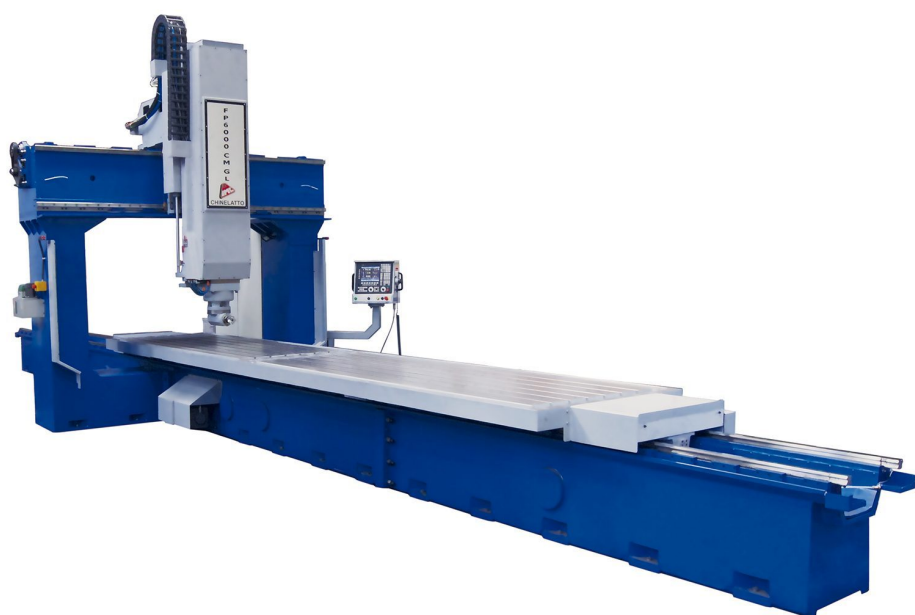
CNC gantry milling machine FP-6000CM x 2200 mm (86.6 in) - with enclosure
