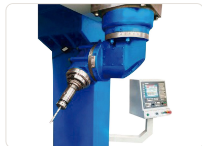
Optional accessory — Sub cylinder head multi angular, with manual positioning
