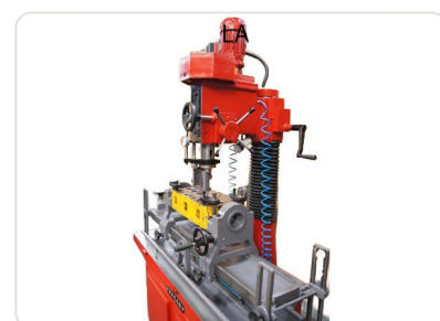
FRECAB Chinelatto valve seat milling machine — general view of machine with tilting table
