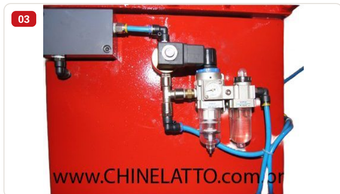
Detail — Pneumatic system with filter regulator for compressed air on FRECAB milling machine - view 1/2
