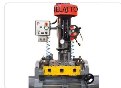
FRECAB valve seat milling machine Chinelatto — front view with tilting table, control panel and 1.5hp motor
