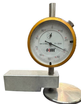
Optional accessory — Device with dial indicator to check valve seat height
