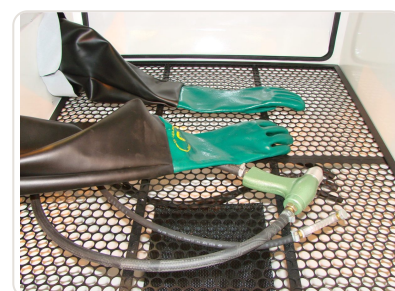
Standard accessory — Internal chamber of JA-900 sandblaster with protective gloves and blasting gun
