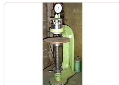
Benchtop hardness tester: - Used to measure material hardness (HB)
