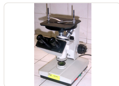
Optical Microscope: - Used for metallographic analysis of the material
