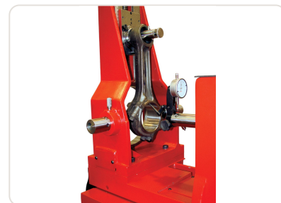
Cast iron connecting rod positioned on MB-125 boring machine with dial indicator for measurement
