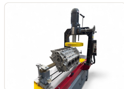
PBC-1200X milling machine resurfacing V8 aluminum cylinder head — view 1
