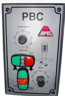
Detail — Control Panel with rotary controls for RPM and table speed of PBC-1200X milling machine
