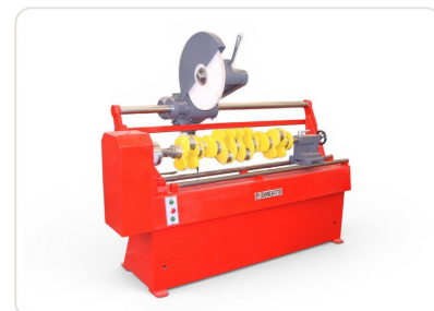
PV-1500 Chinelatto crankshaft polisher with 3hp motor and Ø15.7x59 inch (Ø400x1500mm) capacity
