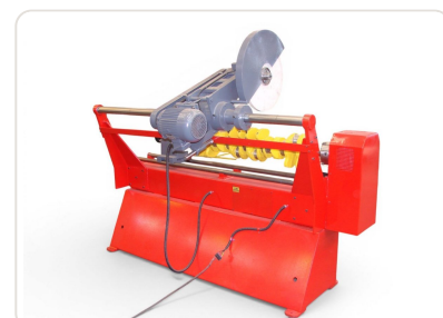
Crankshaft polisher PV-1500 Chinelatto Ø16x59 inch (Ø400x1500mm) with 3hp motor and Ø20 inch (Ø500mm) polishing disc
