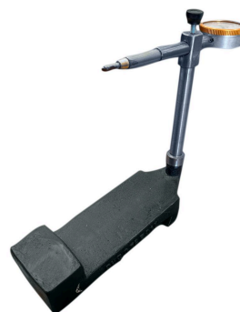
Standard accessory — Crankshaft centering fixture with dial indicator
