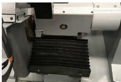
Detail — Grinding wheel slide protection with metal accordion bellows for RVC-1000M grinder
