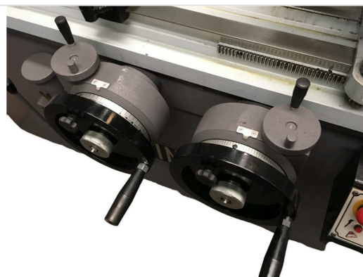
Detail — Manual movement handwheels in cast iron with handles for feed control of RVC-1000M grinder
