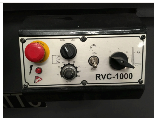
Detail — Variable rotation speed control panel of RVC-1000 grinder with speed controls and emergency stop
