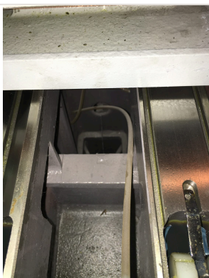
Detail — Cast iron bed with internal ribbing of RVC-1000M grinder, showing linear guides
