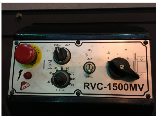
Detail — Control panel with speed variator for RVC-1500MV grinder, emergency button and rpm controls
