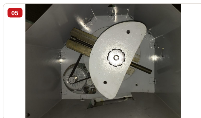
Detail — Grinding head advance and counterweight system with manual micrometric handwheel
