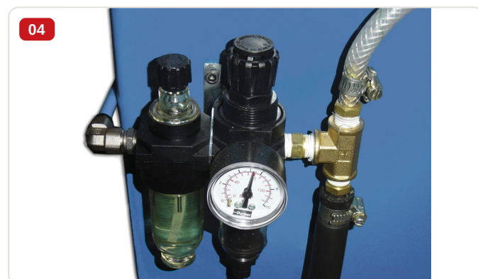
Detail — Pneumatic system with Parker regulator, pressure gauge and air filter for 87 PSI (6 bar) compressed air supply
