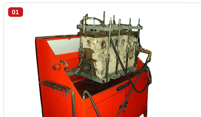
Detail — TESTRIM pressure tester with mounted cylinder head for crack and leak detection
