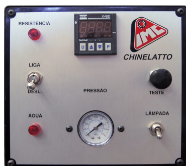
Detail — Control panel of TESTRIM pressure tester with digital display, pressure gauge and controls
